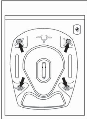
For this reason, transport safety screws shall be loosened by being rotated in counter-clockwise using an appropriate wrench.
