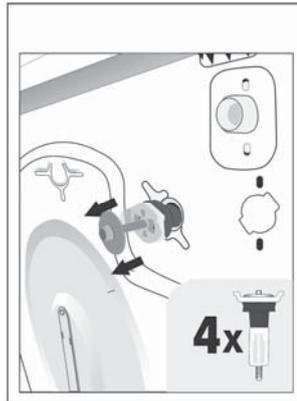
Fit the plastic transport screw taps delivered in accessories bag to the places where transport screws have been removed.
